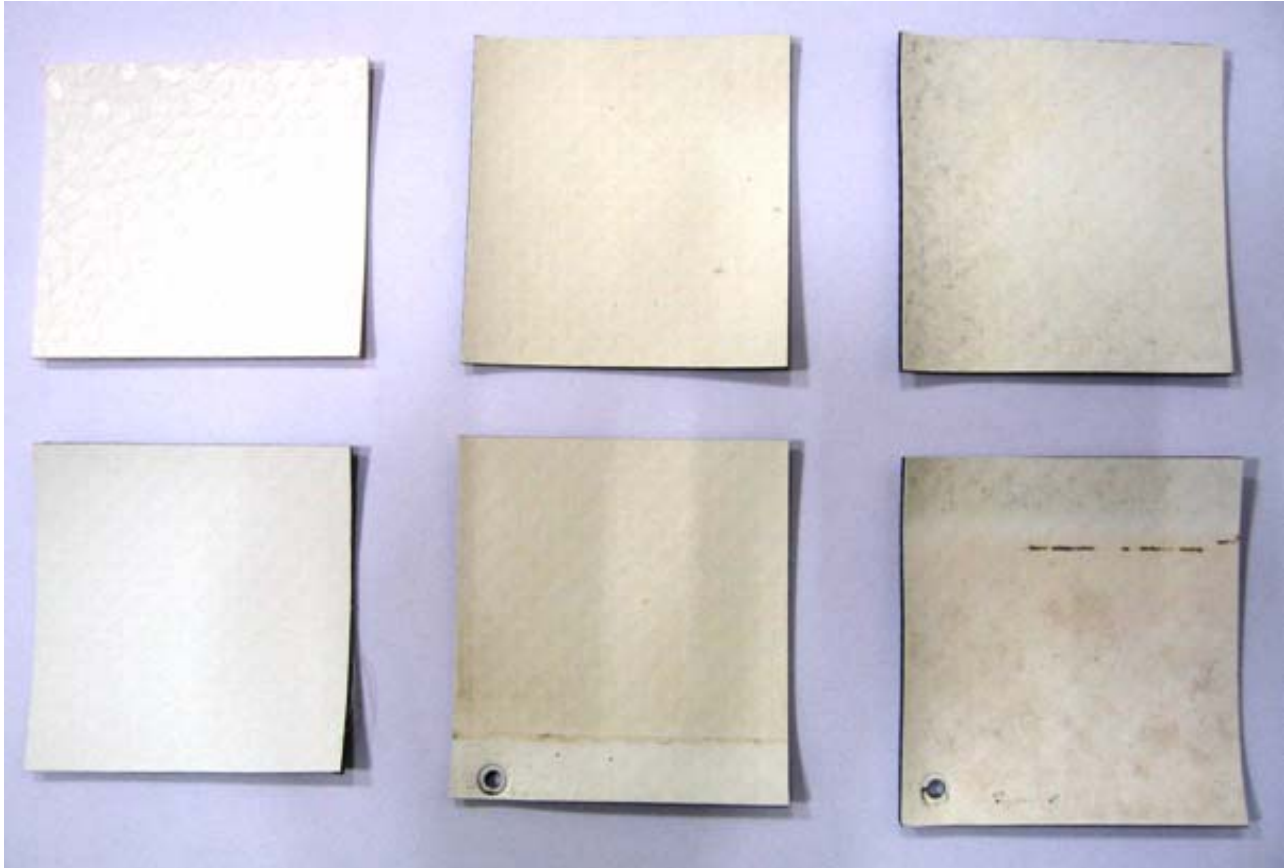
Figure 4.1. Sample set A (ALKORPLAN F 35276 WHITE – ALKORBRIGHT): representative sample (upper left); sample set B (RENOLIT ALKORPLAN F WHITE): non weathered sample (lower left), samples weathered in Arizona (middle) and samples weathered in Florida (right).
