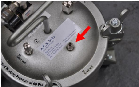
Follow the same method – as described in previous paragraph – after unscrewing the 4 wing nuts. After the filling just connect the air hose, the set pressures stay as they were before.
