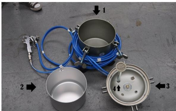
Fill the inner bucket (2) with adhesive, avoid dirt which may be on the top of the adhesive container falls into the bucket.
