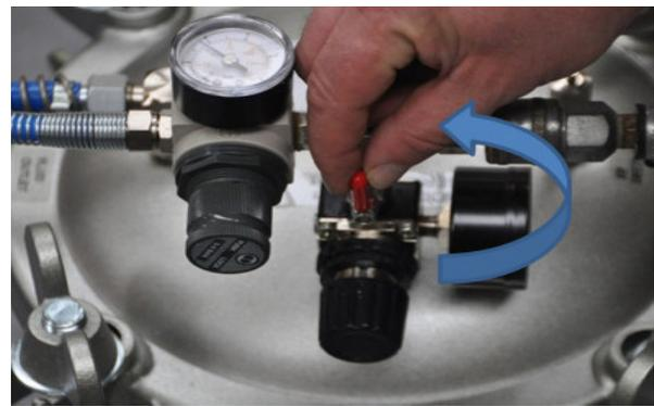
Adjust the pressure on the glue (1) to approx. 4 bar (3) & the spray pressure to the gun (2) at 5,5 bars (4).
